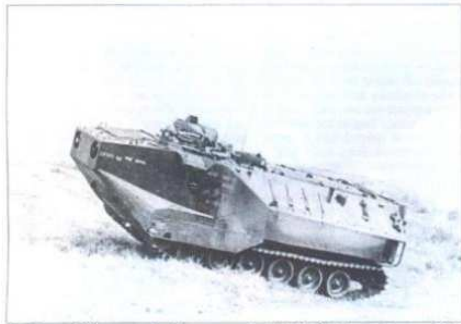
The first vehicle to use the Gleasman steering gear will be the 26-ton LVTP7, the advanced amphibious landing vehi-
