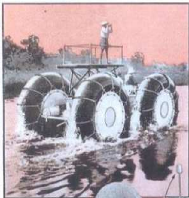
The "marshbuggy" afloat. The giant tires provide buoyancy, and cleats give traction in the water.
