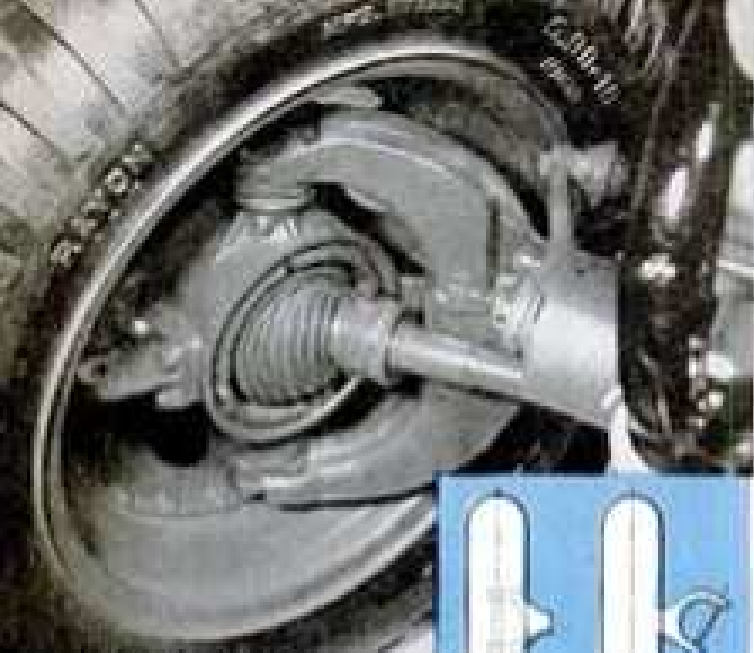
FRONT WHEELS are pivoted on vertical kingpins centered inside the hubs.
