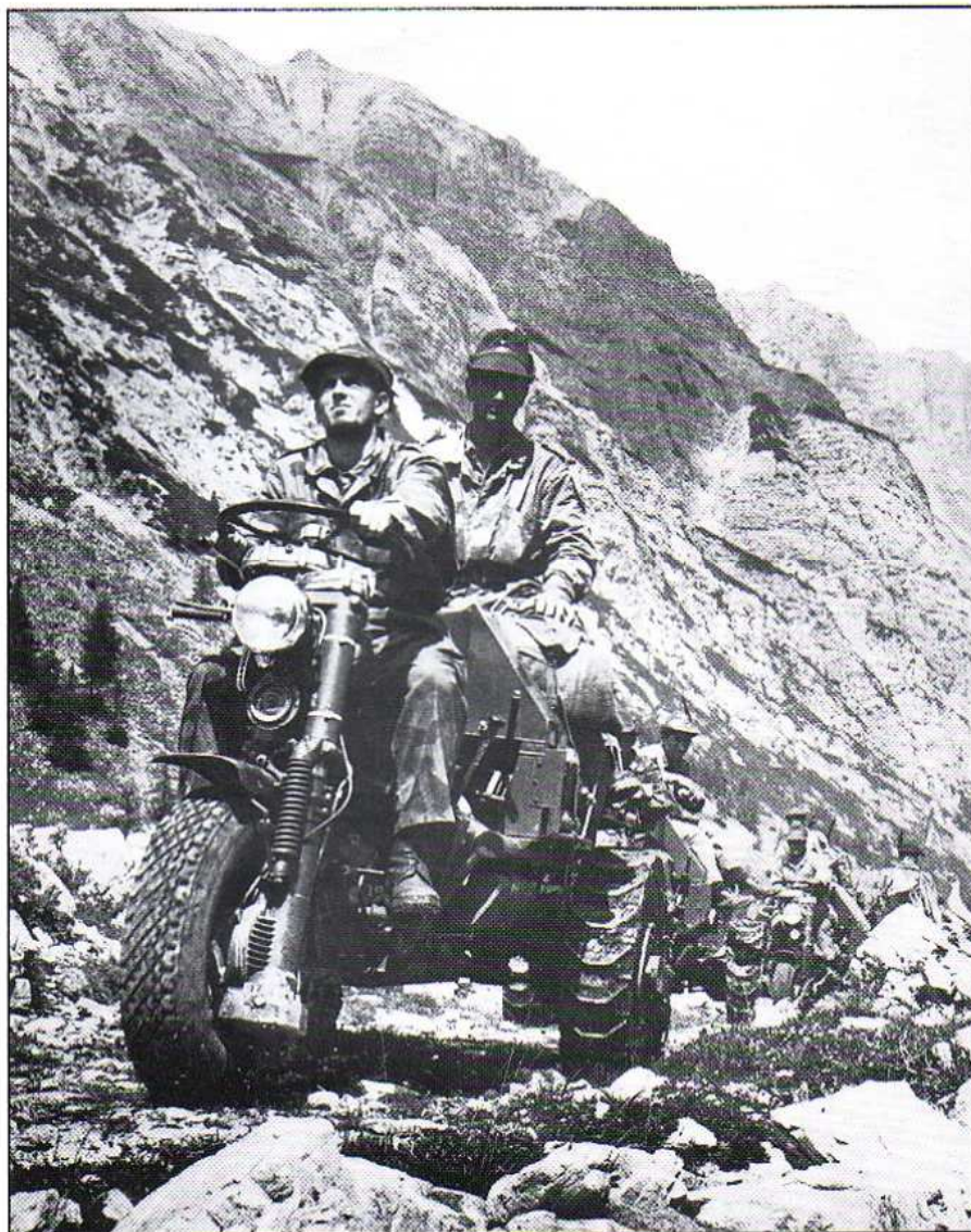
Pilot models — recognisable by different steering column and other details — under test. Upper left picture shows reduced rear track; this narrowing down (and vice versa) could be accomplished on the move, within 25 metres travelling distance.
