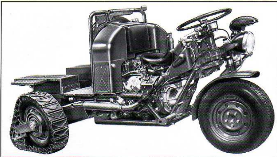
By lowering the rollers and installing the overall tracks the Mulo becomes a half-track. Driver's back rest is in fuel tank recess. The machine was an overkill, expensive and unsafe.
