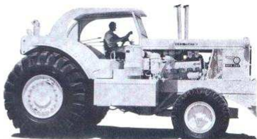
Above: The 1961 M-R-S 250 was spectacularly large, weighing in at 64,340 lbs and having a 1,710 cubic inch Cummins V-12 providing a top speed of 34mph in ninth (top) gear.
