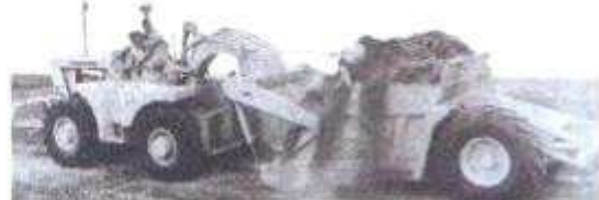
M-R-S Hancock Elevating Scraper Combination Features Four Wheel Drive-12 Yard Capacity
