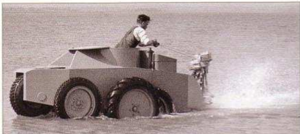
It was described as being amphibious but the driver had to lean out of the hull like this to start the auxiliary outboard motor - speed in water was at best 1 knot. (IWM, H19443)
