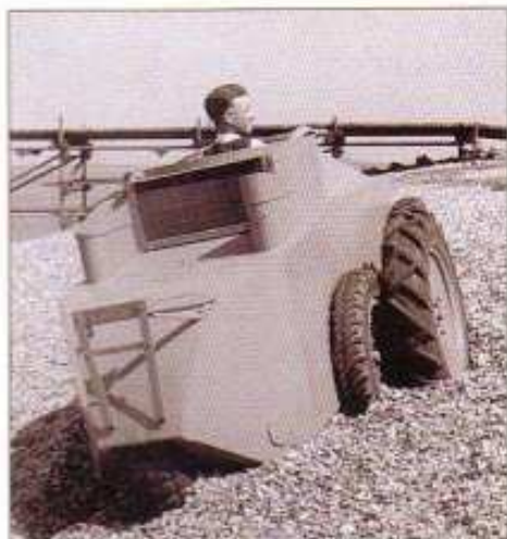
Since the driver is not evident in other views, one has to conclude that, in this case, the Scorpion has been defeated by the loose shingle and that the driver is attempting to extricate himself from the hull. (IWM, H19432)
